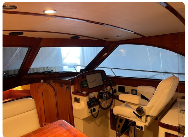
{1} Lower helm station
