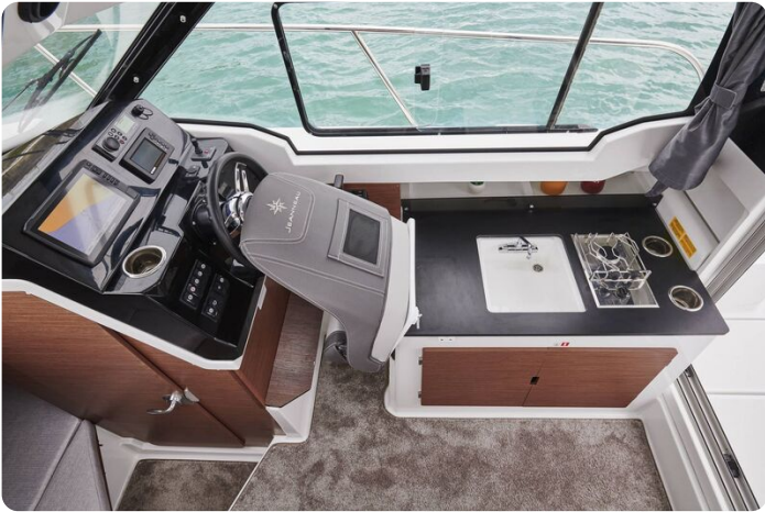
Jeanneau Merry Fisher 795 Series 2 - helm seat folds forward for easier access to galley
