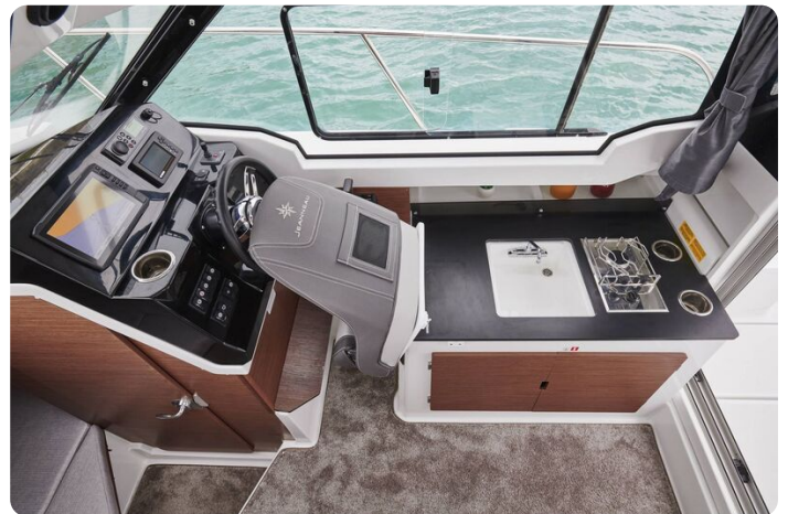
Jeanneau Merry Fisher 795 - helm seat folds forward for access to galley
