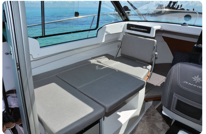
Jeanneau Merry Fisher 695 wheelhouse boat - wheelhouse saloon converts to berth
